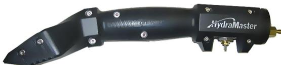
**Figure 3-3. Remove All Screws on Tool**
