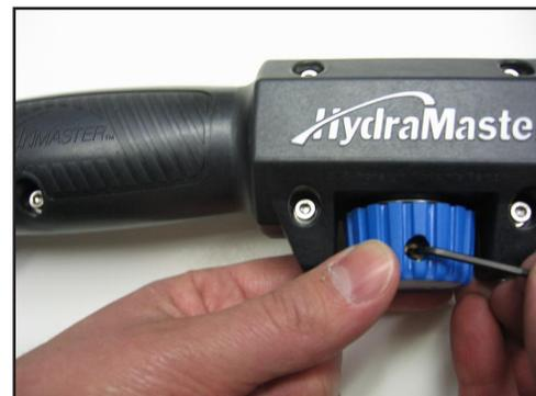
**Figure 3-2. Remove Solution Control Knob**
