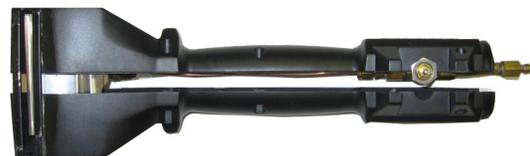
**Figure 3-4. Separate Tool in Half**
