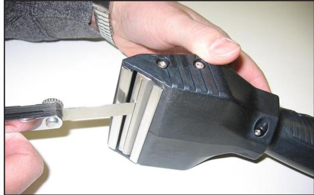
**Figure 3-6. Clean the Solution Bar Jet**
